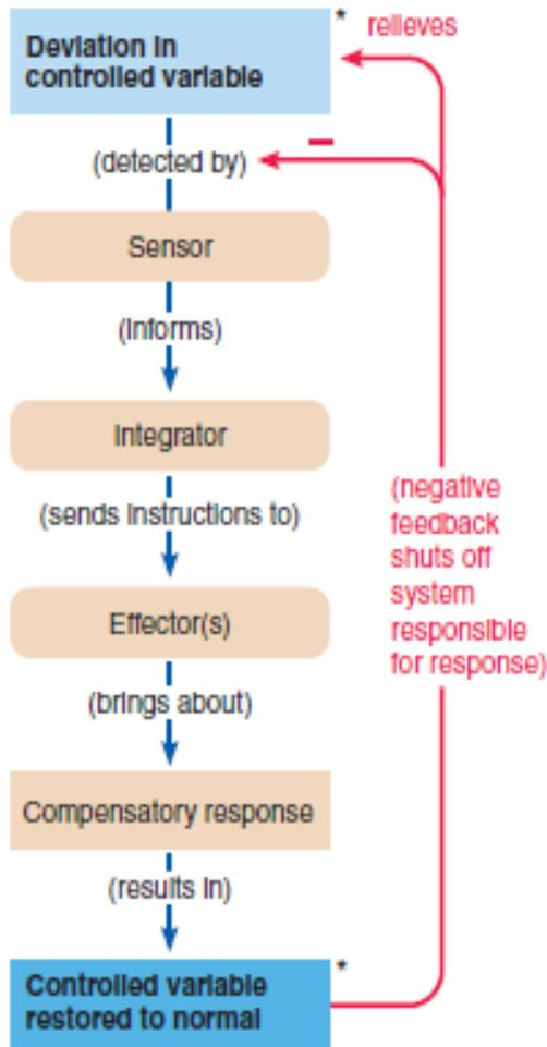
(a) Components of a negative-feedback control system
